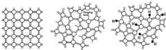
Figure 4: Schematic structures of crystalline silicon, amorphous silicon, and amorphous hydrogenated silicon
