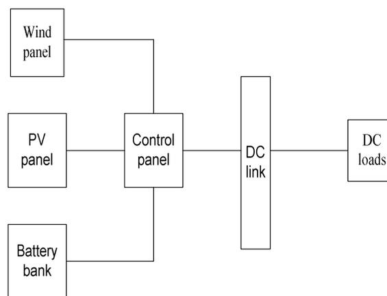
Fig. 1 Hybrid wind-PV-battery system.
