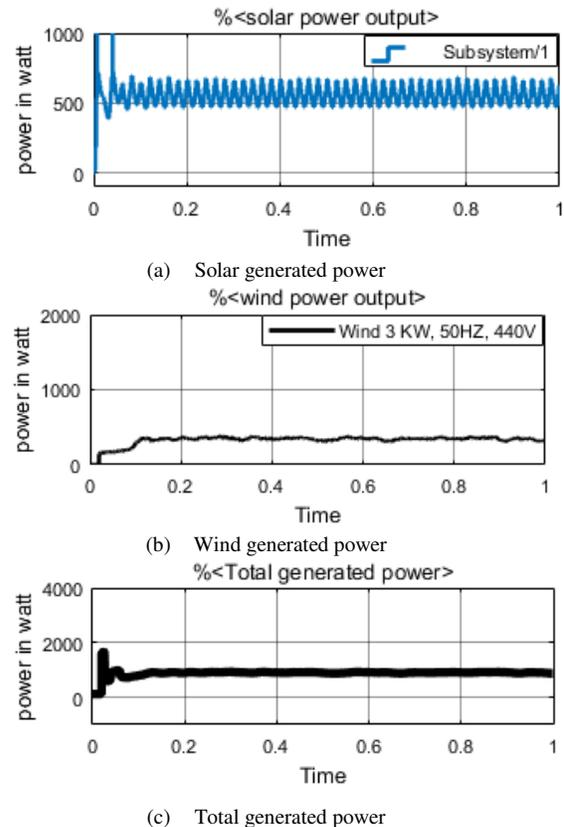
Fig. 7 Waveform of solar generated power, wind generated power and total power.
