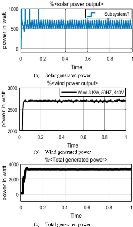
Fig. 6 Waveform of solar generated power, wind generated power and total generated power.
