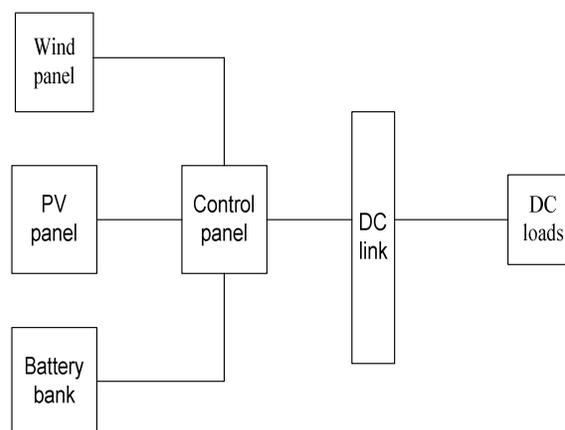
Fig. 1 Hybrid wind-PV-battery system.
