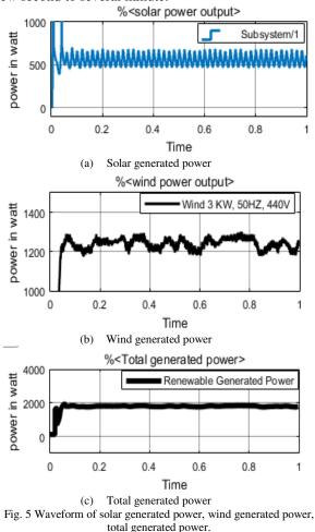
Case : Solar irradiation at 1600W/m<sup>2</sup> and wind speed same 12m/s
