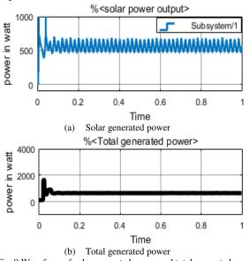
Fig. 9 Waveform of solar generated power and total generated power. Case : Solar irradiation at zero  $W/m^2$  and wind speed zero m/s
