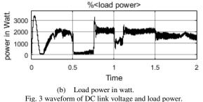
Case : Solar irradiation at 1000W/m<sup>2</sup> and 13m/s wind speed
