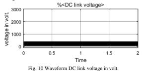
Case :- Load is zero and generated power is continuous
