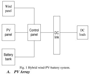
PV array is not a single cell it is a combination of number solar cell in series and parallel connected mode and module is a combination of series and parallel connected cells. Operating point of PV-module determined by DC voltage of the cell and PV array output depends on isolation level, and affected by the temperature.
