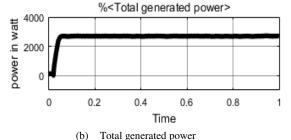
Fig. 8 Waveform of wind generated power and total generated power. **Case : Solar irradiation at 1000W/m<sup>2</sup> and wind** speed at zero m/s
