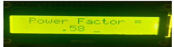
Fig. 3: Initial Power Factor for Inductive Load
