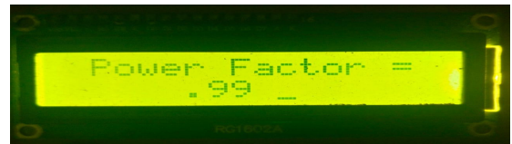
Fig. 4: Final Power Factor for Inductive Load
