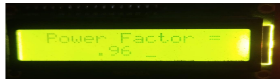
Fig. 5: Initial Power Factor for Resistive Load
